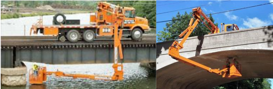
Example of a Specialized Vehicle that Allows Up-close Inspections
