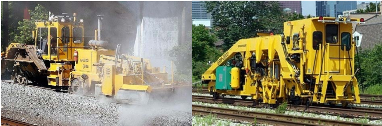
Figure 1: Examples of Track Equipment used by Metro-North. A ballast regulator (left) spreads the stone and distributes it evenly. A ballast tamper (right) is used to pack the ballast under tracks to make the tracks more durable.
